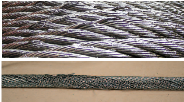
This is what happens when spooling on multiple layer drums was not properly tensioned.
