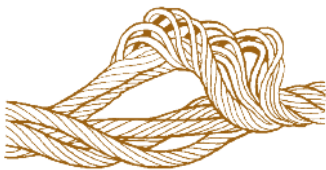
Bird Cage forced through a tight sheave.
