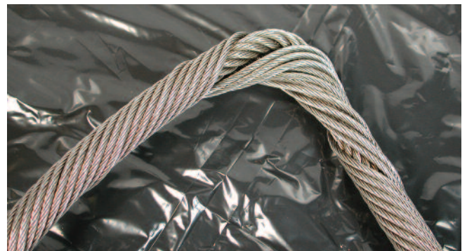
Actual example of a rotation resistant wire rope which was forced to run in too tight sheave grooves. Result is so called 'core popping'.
