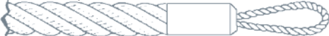
Wire Rope welded together. Danger of the weld breaking when bent around sheaves.
