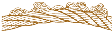
Protruding Core because of shock loading, torque build-up during installation, tight sheaves, or incorrect rope design.
