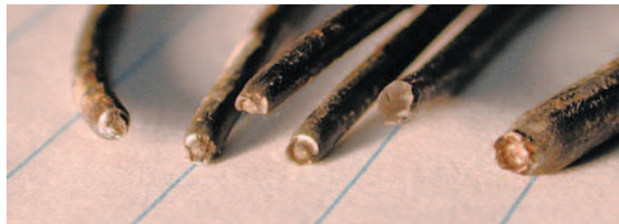
Condition of core under that same single valley break. Note the extreme notching of individual wire and the countless wire breaks. Such a condition is hidden under just a single (1) valley break !
