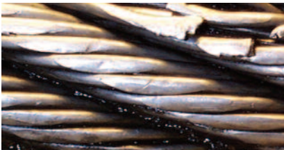
Peening and subsequent wire break caused by high fleet angle and rope vibration.
