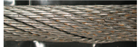
Crown wire breaks on a Python® Lift non-rotating wire rope
