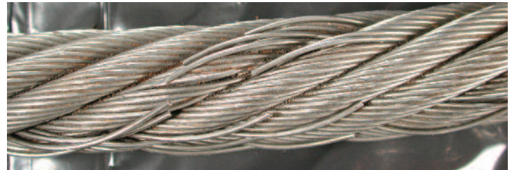
Example: Valley wire breaks on a 8-strand overhead crane wire rope
