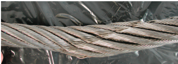
Actual example of a wire rope which jumped out of the sheave. Note the imprint of the sheave flange.
