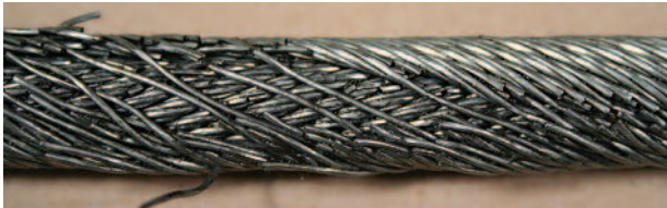
This is what happens when spooling on multiple layer drums was not properly tensioned.
