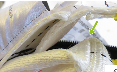
• No tearing of the energy absorber
