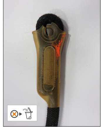
• Damaged plastic sleeve
