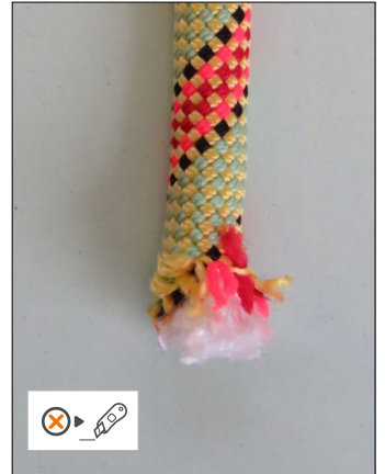
• Damaged rope end
