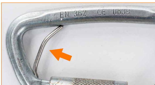
Connector with deformed ACL bar.
