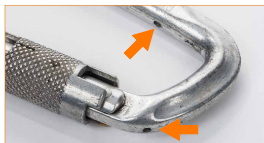
Connector with missing bar.
