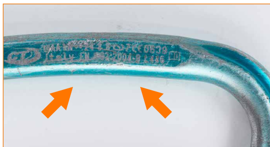
Connector's markings not completely legible.
