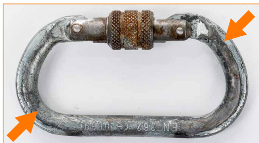
Connector with clear incision/cut on body.
