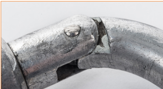
Connector with worn-out pin.
