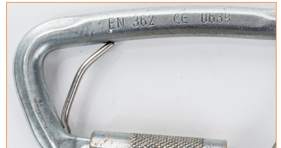
Connector with deformed ACL bar.
