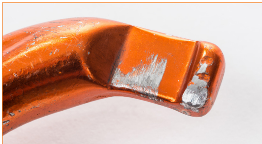
Connector with damaged nose because of the misalignment of the lever.
