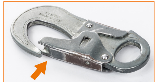
Oxidation on connector prevents closing catches functioning correctly.
