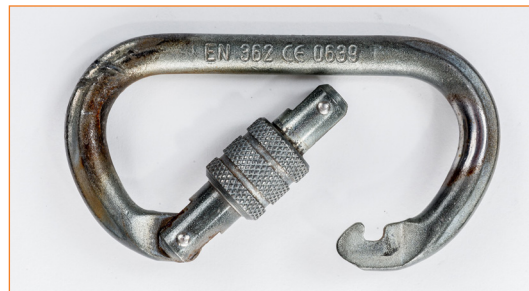
Connector with completely blocked lever or with damaged / missing spring
