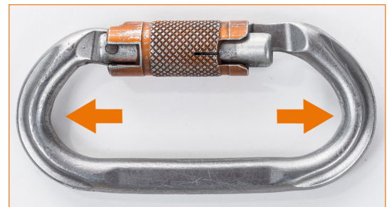
Connector with screw-up locking sleeve extremely deformed due to incorrect use.
