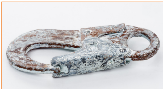
Steel connector completely corroded after long exposure to saline environment.
