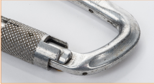
Connector with missing bar.
