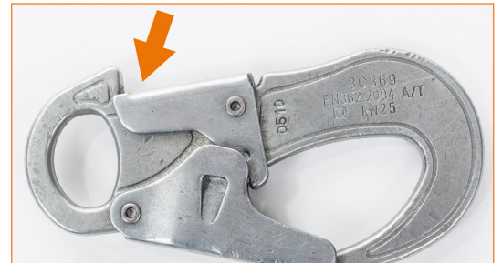
Double-lever connector whose rear safety lever doesn't return automatically into position.
