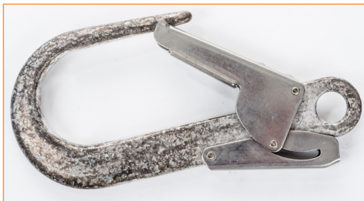
Double-lever connector with clear signs of corrosion.
