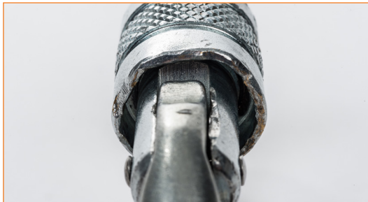
Connector with heavily damaged screw gate.
