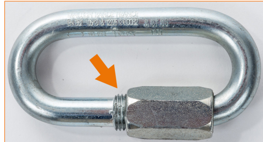
Quicklink with the screw-up sleeve screwed beyond allowed limit.
