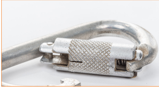
Connector with gate that remains open.
