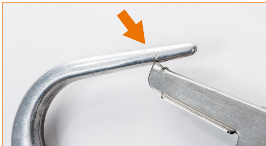
Connector with catch no longer aligned with body due to major torsion loading.
