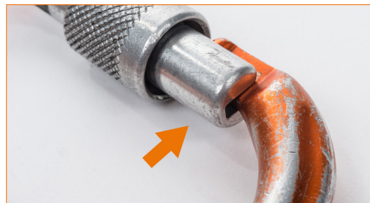
With gate in closed position, gate remains slightly open with play towards correctly-closed position.
