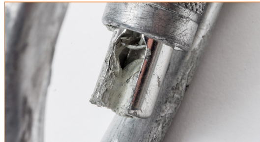
Connector with material inside holes and cracks. ⚠️ Clean the device with compressed air and soap and water. If the problem is not resolved, scrap the device.
