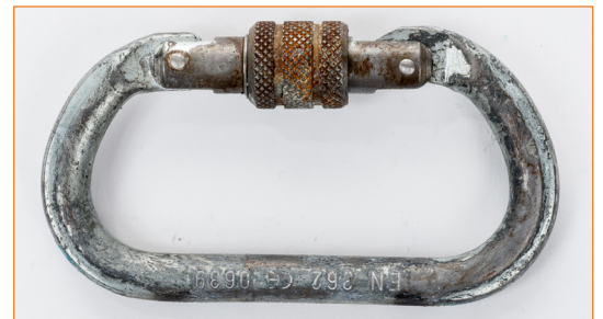
Connector with clear incision/cut on body.
