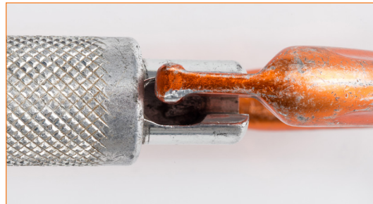
Connector with misaligned lever from the body.
