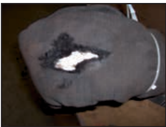
Exposed load bearing yarns
