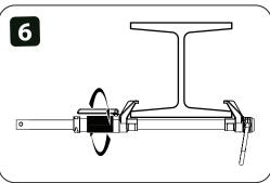
6. Hand tighten nut as much as possible by turning clockwise.
