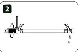
2. Fully loosen nut by turning counterclockwise.
