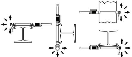
\*Note: Placement at or below a user's working height requires integration of a compatible ANSI Z359.18 Type T shock-absorbing lanyard that does not allow user to extend more than 6 feet (1.8m) (in any direction) from the anchorage connector before shock absorber is activated. Beam anchor must be attached to I-beam flange facing the user (top flange if above, bottom flange if below, etc.).
