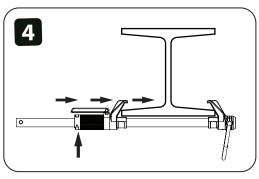
4. Press lock button and slide adjustable paw to tightest notch to capture I-beam flange.
